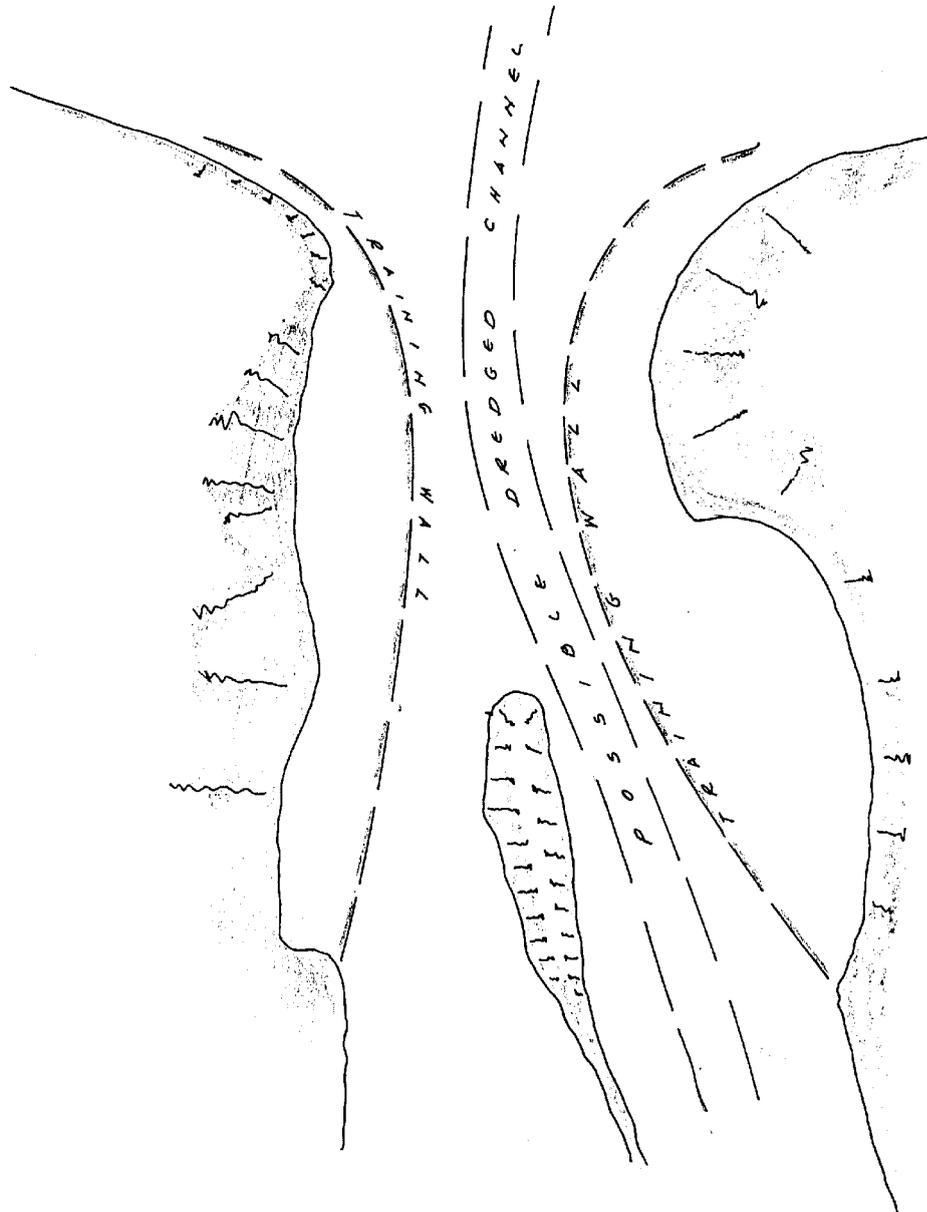
FIG. 4 POSSIBLE ALIGNMENT OF TRAINING WALLS (N.T.S)
