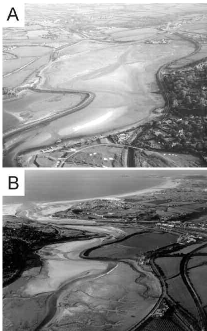
Figure 2. Oblique air photographs of the Hayle Estuary area. (a) View southwest towards the Hayle branch of the estuary. The mine waste contaminated sediments form the intertidal areas at the head of the estuary. (b) View north showing Carnsew Pool, constructed in 1834 as a means of maintaining the narrow active channel which flows out into St. Ives Bay.
